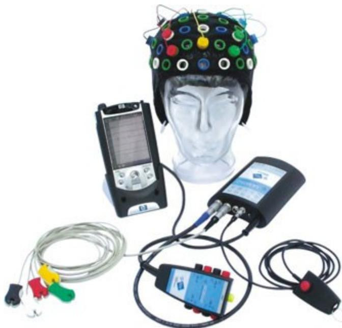
**Figure 2 An electroencephalogram (EEG) based noninvasive brain-computer interface from Guger Technologies OEG (<http://www.gtec.at>)**
