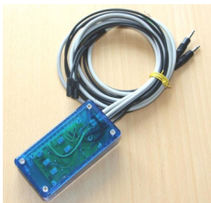
Interface between two SIE sensors and the Octopus.
