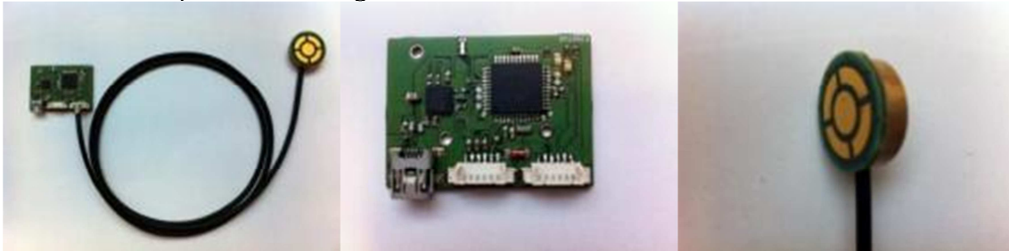
Figur 3. Capacitive sensor with dongel
