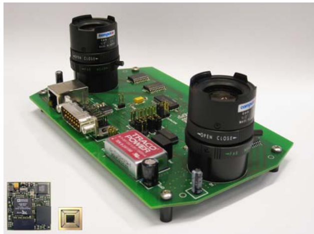
Figure 1: Image of the event-driven stereo vision system. In the lower left corner the DSP Bf537 and the sensor chip are shown. The DSP is mounted on the back of the board.
