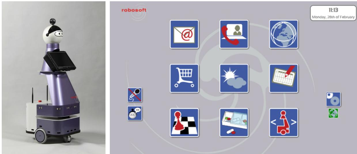
**Figure 1: RobuMATE prototype and HCI/HMI main menu on Touchscreen PC (Tablet PC)**
