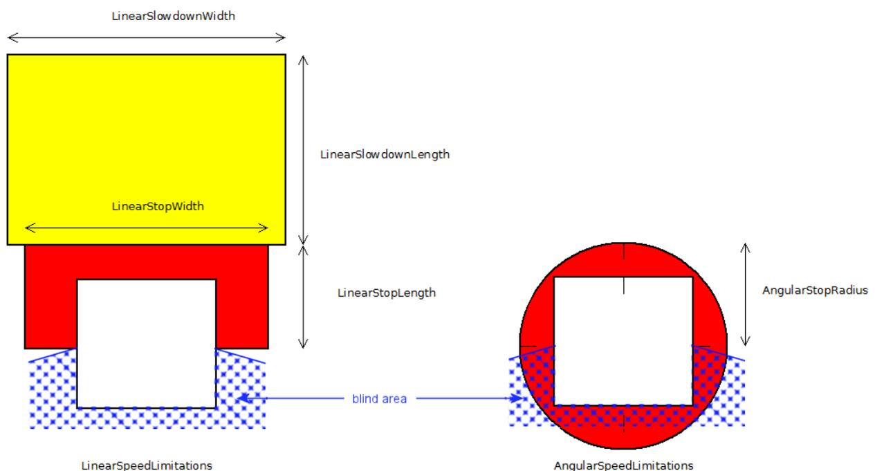
**Figure 5: the collision avoidance settings (stop zones and simplified blind area)**
