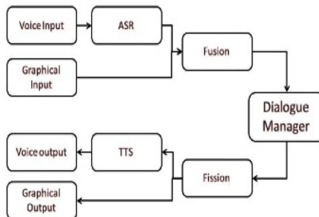
**Figure 25 Multimodal approach using fusion and fission processes to combine speech, tactile and graphical signals**
