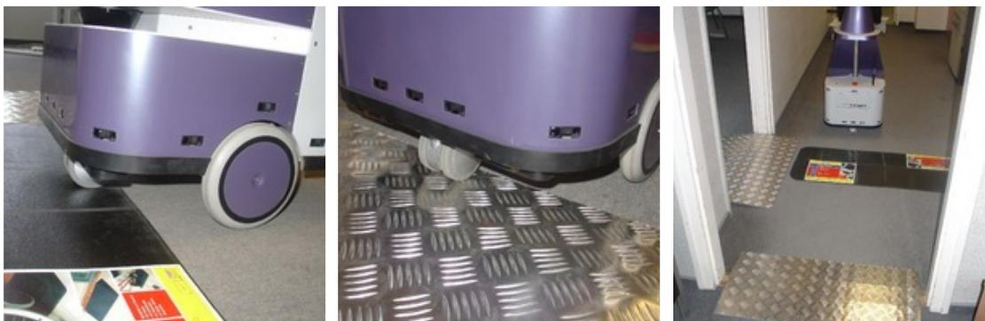
Figure 2: tests for passing of ramps and steps done at BME
