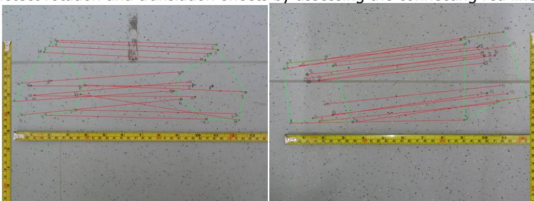
**Figure 4: Position hit patterns for repeated positioning between two PoIs**
