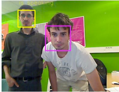
**Figure 29 Speaker detection based on lips movements**
