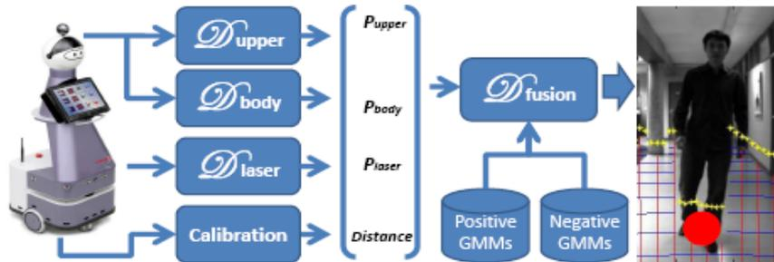
**Figure 17 Synopsis of the developed human detection system.**
