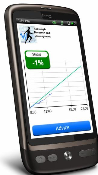
**Figure 5:** the PDA activity monitoring and feedback application, running on an HTC Desire (Android 2.2), showing the activity graph of the patient (blue), plotted over the desired reference activity graph (green). The status panel shows the current deviation from the reference line in percentage points.
