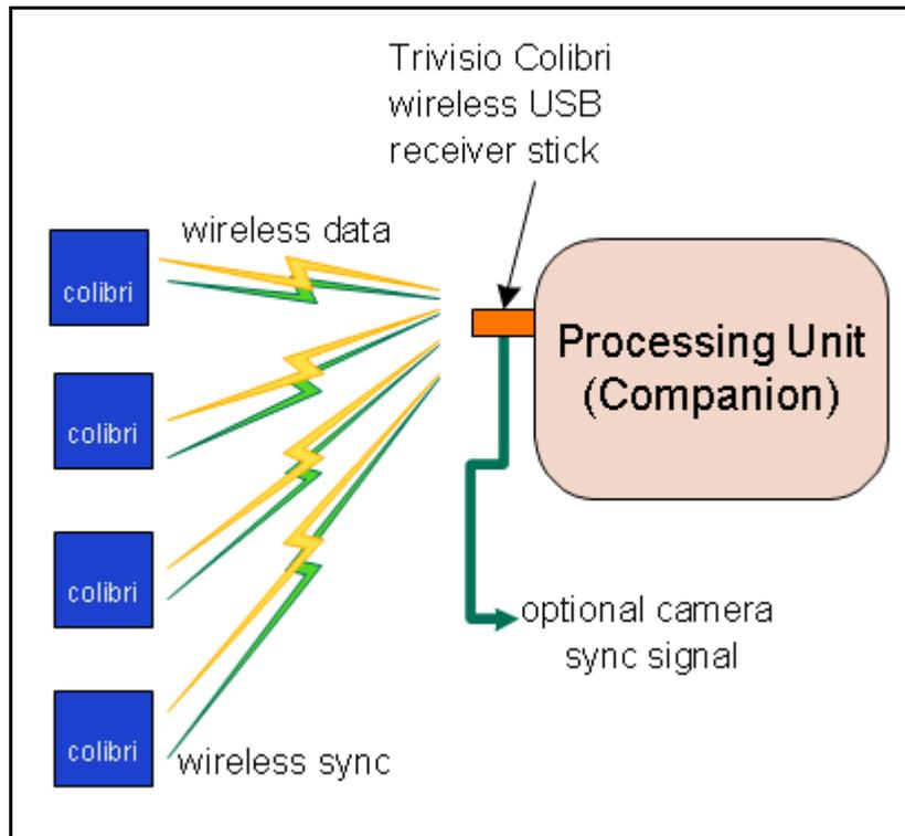
Figure 5: Wireless IMU sensors sync
