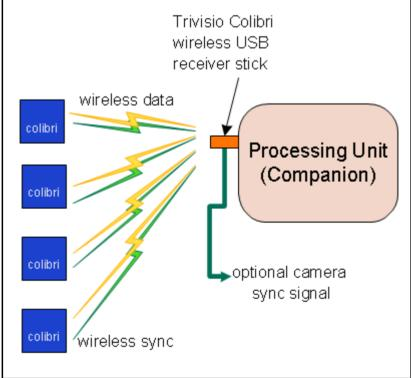
Figure 5: Wireless IMU sensors sync
