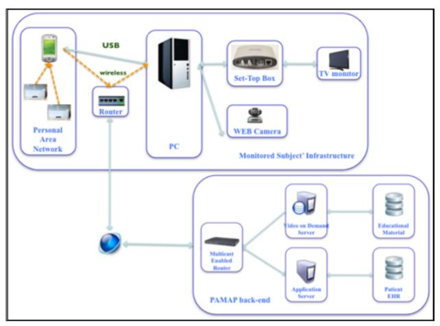
Figure 2: PAMAP Measurement Component Interaction Diagram
