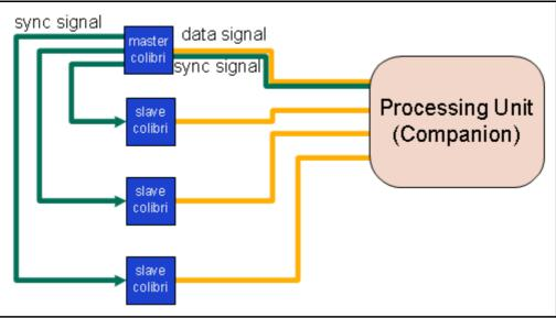
Figure 4: Wired IMUs with wired sync possibility.
