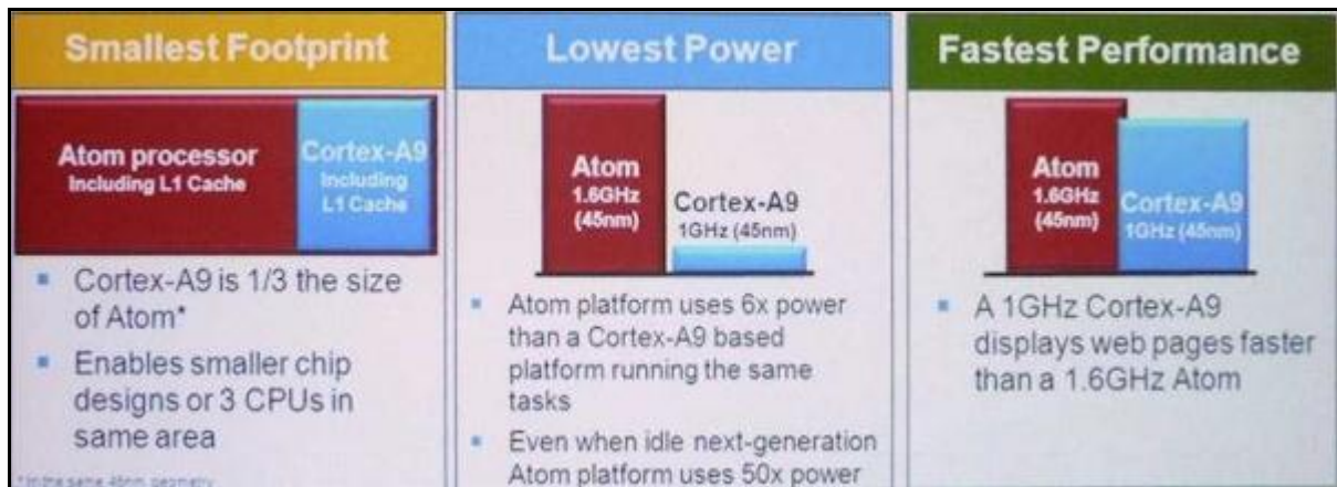
Figure 11: RISC/ARM vs. Intel® Atom™ (Source: PC Watch - http://pc.watch.impress.co.jp )
