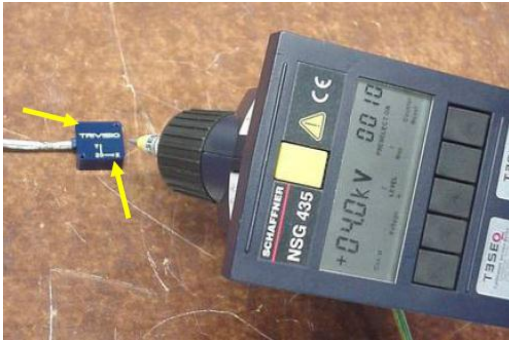
Figure 4: Colibri sensor in ESD test
