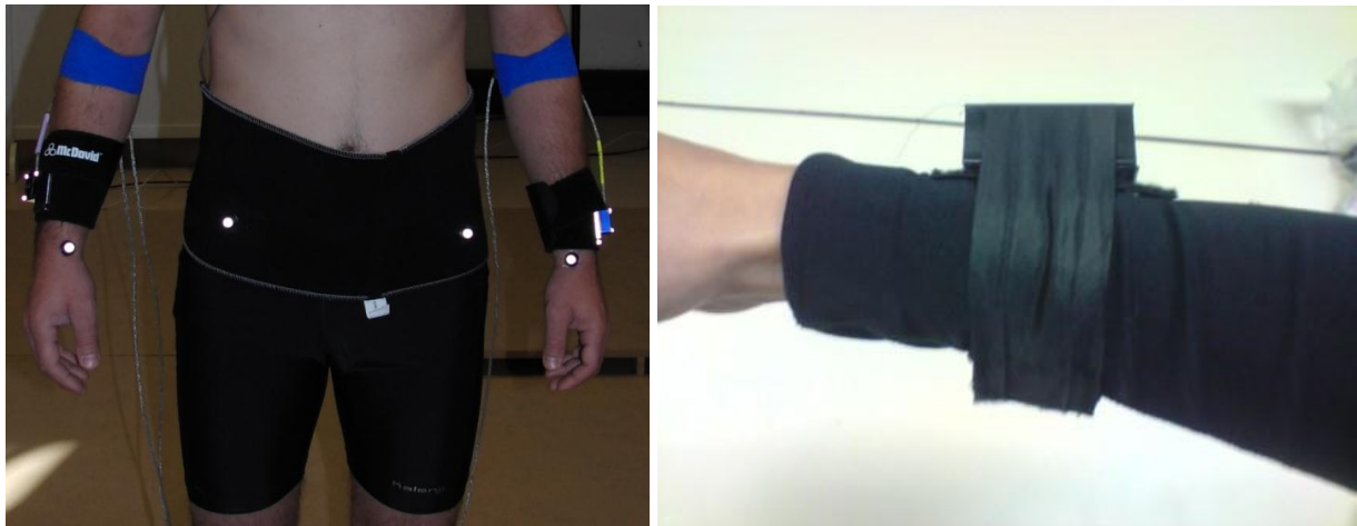
Figure 15: Sensor fastening based on bandages (on the left) and on a body suit and velcros (on the right).
