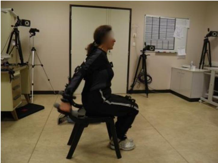
Figure 3: Three of the 8 Vicon cameras around the subject.
