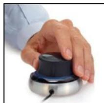
Figure 27.3D Mouse: 3D Connexion – Space Navigator
