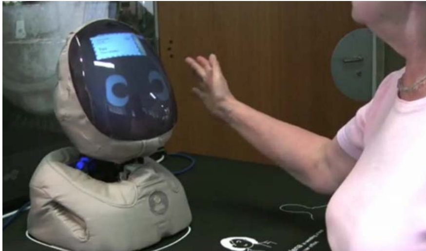
Figure 1: The Kompott prototype, its whole face is represented by a touchscreen. Touching the head itself accounts as user input, also.
