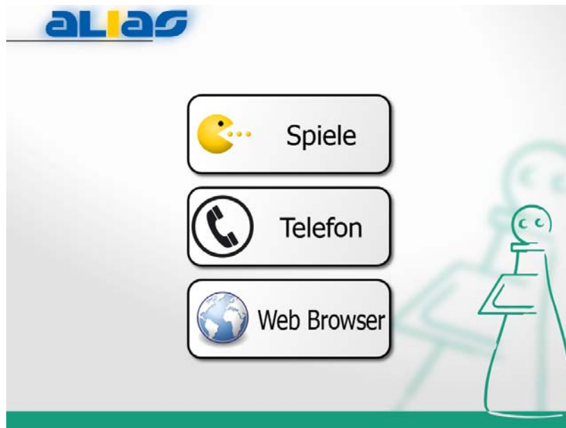
Figure 2: The GUI's main menu. The Button "Spiele" brings-up the games sub-menu, while "Telefon" starts the telephone application, and "Web Browser" runs the integrated web-browser.
