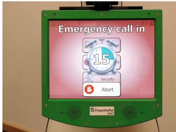
Figure 2: The ALIAS system uses the display unit to notify the user about an eminent emergency call.
