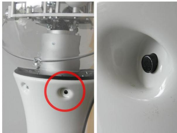
Figure 3: The robot's revised microphone, located at its neck.
