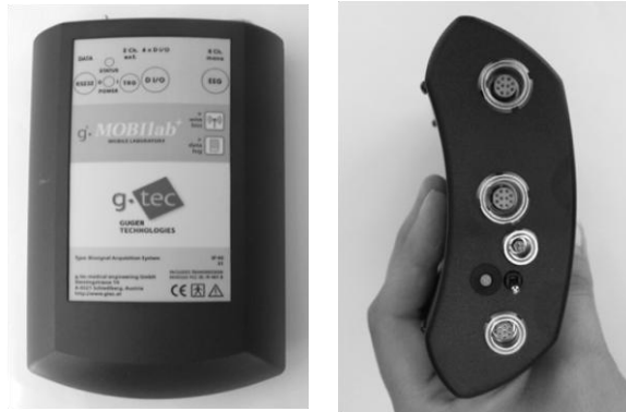
Figure 8: Portable channel EEG amplifier g.Mobilab+ with Blue-Tooth based connection
