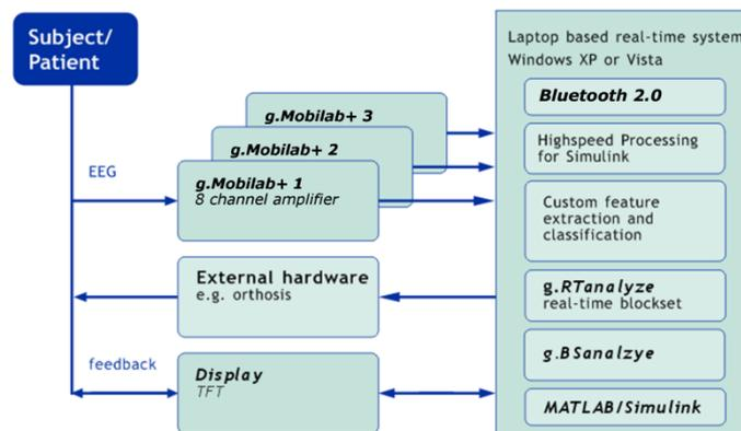
Figure 9: BCI architecture with Matlab/Simulink
