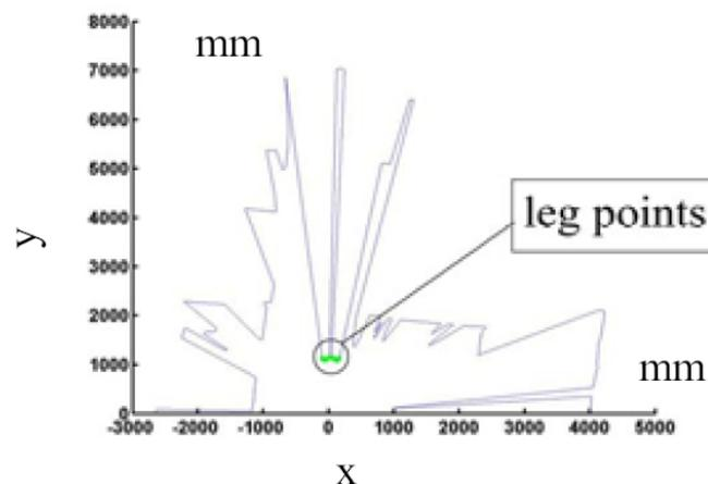
Figure 3.4: Image from [24]. Here, a laser scan, including two legs, is shown. The mean position of both legs is used to control the robot.
