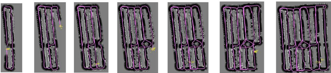
Figure 2.4: Our iterative on-line approach on learning a map. The driven path and the corresponding map is estimated by a particle filter. In this example (from [16]) a home store is shown.
