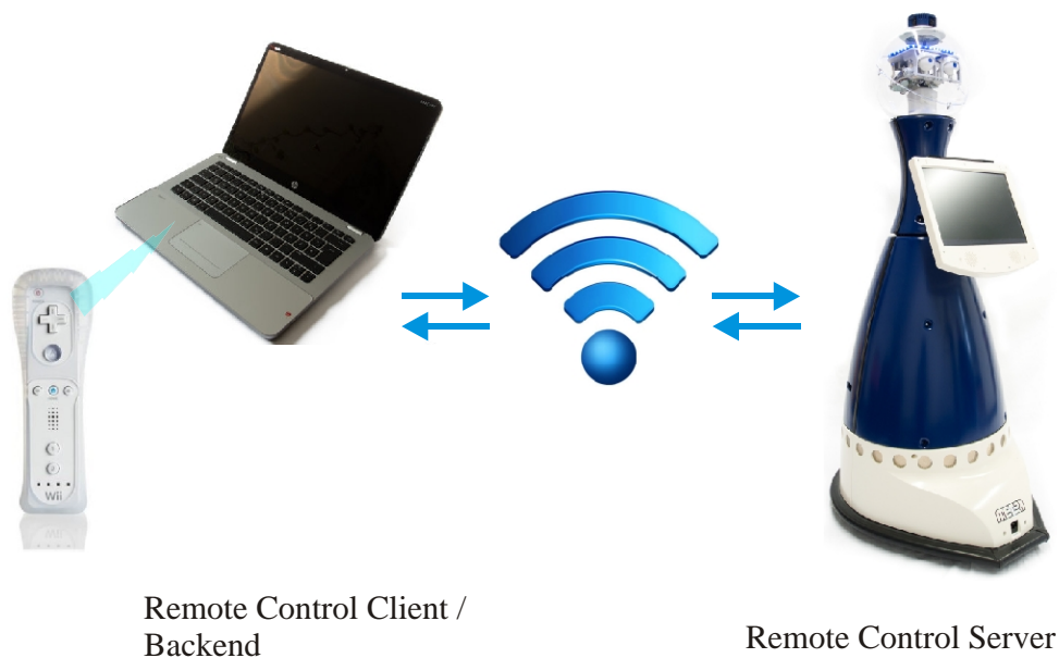
Figure 5.2: the network configuration during the remote control process. The robot is steerable with the Wii remote controller, which is connected via Bluetooth to the remote client. The client uses a standard TCP/IP connection to the remote server (the robot). Over this connection the wished user speed is transferred from the client to the robot and laser distance data plus video and audio data are transferred from the robot to the client.
