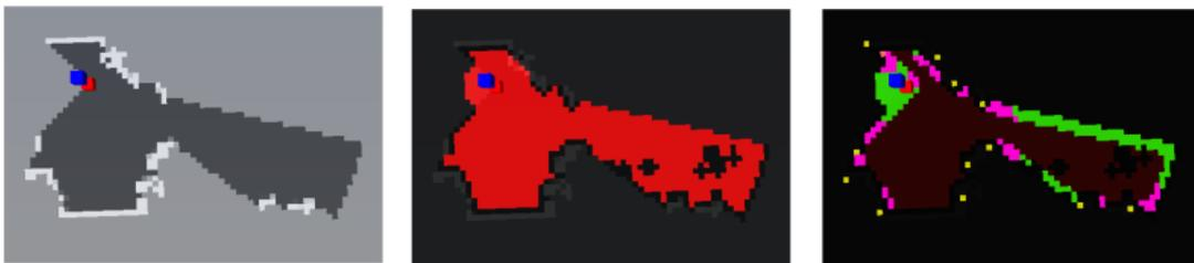
Figure 7.2: The sequence of extracting the next exploration candidate, shown on a small map. On the left the current map is shown (with the robot as a blue and red box). In the middle the reachable cells are shown in red, while on the right side the distinct features are shown in yellow, the edge cells are shown in green, and possible candidates are shown as purple pixels.
