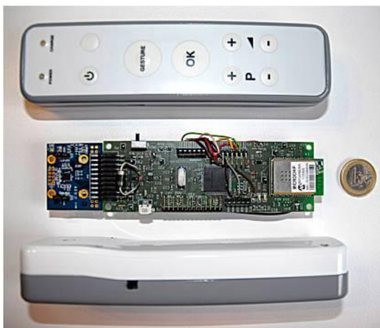
Figure 4: The EasyReach Remote Control's internal electronics
