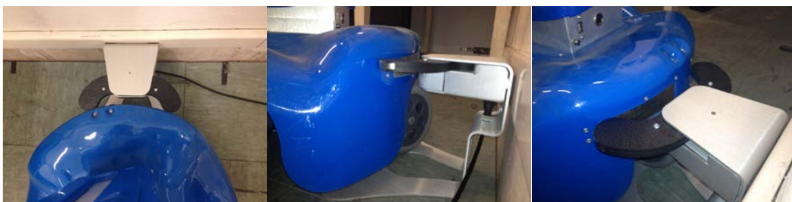
Figure 9 A robot not correctly docked at the recharging station.
