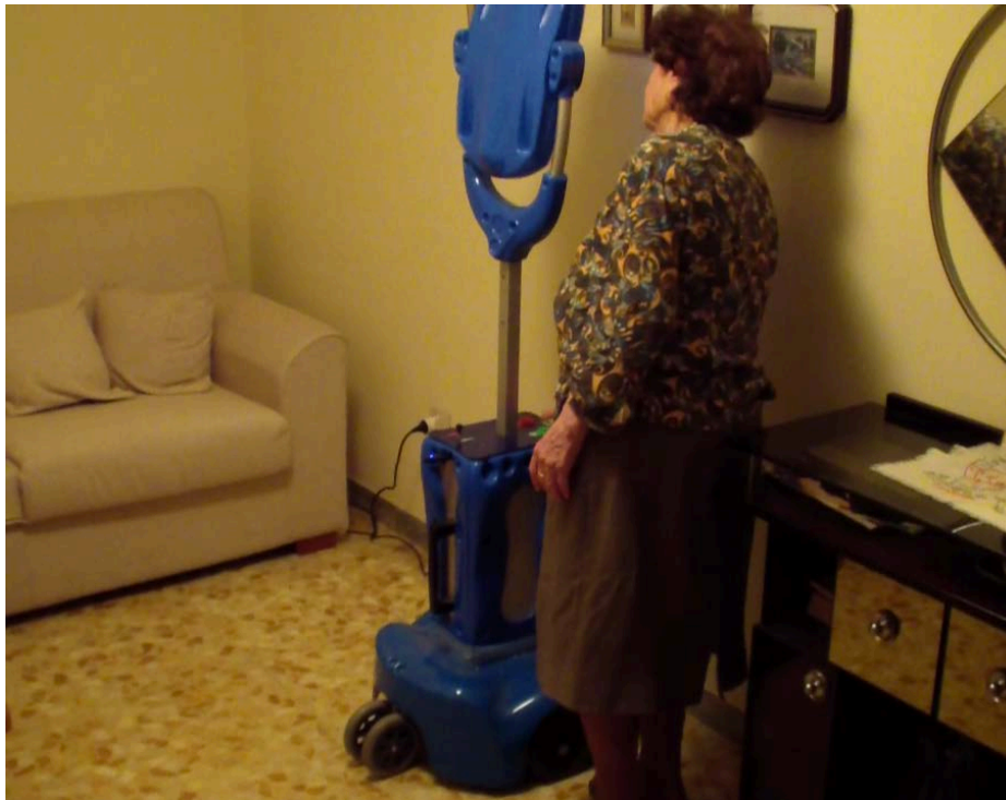
Figure 16 Test site in Italy: Example of problem when answering a call due to the orientation of the robot
