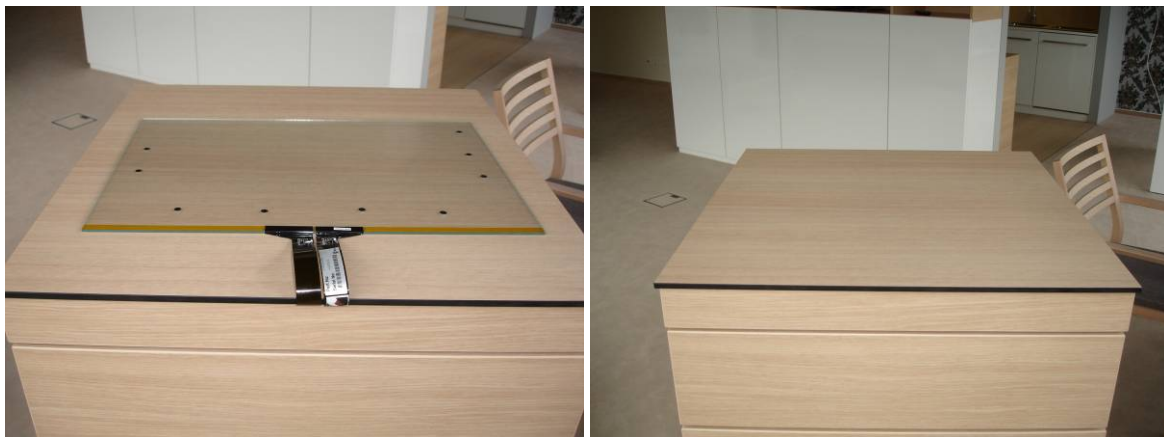
Figure 9: (a) Touch screen for gesture recognition (b) Integration under the wood panel
