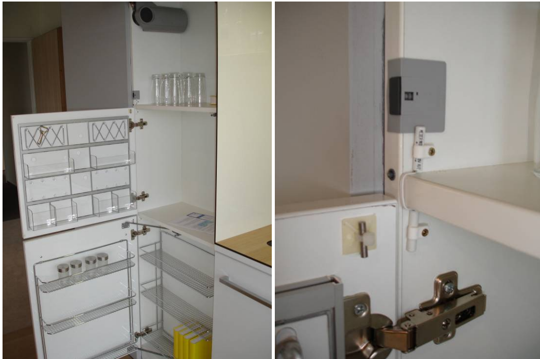
Figure 5: (a) Sensors in the cabinet door (b) Detailed view
