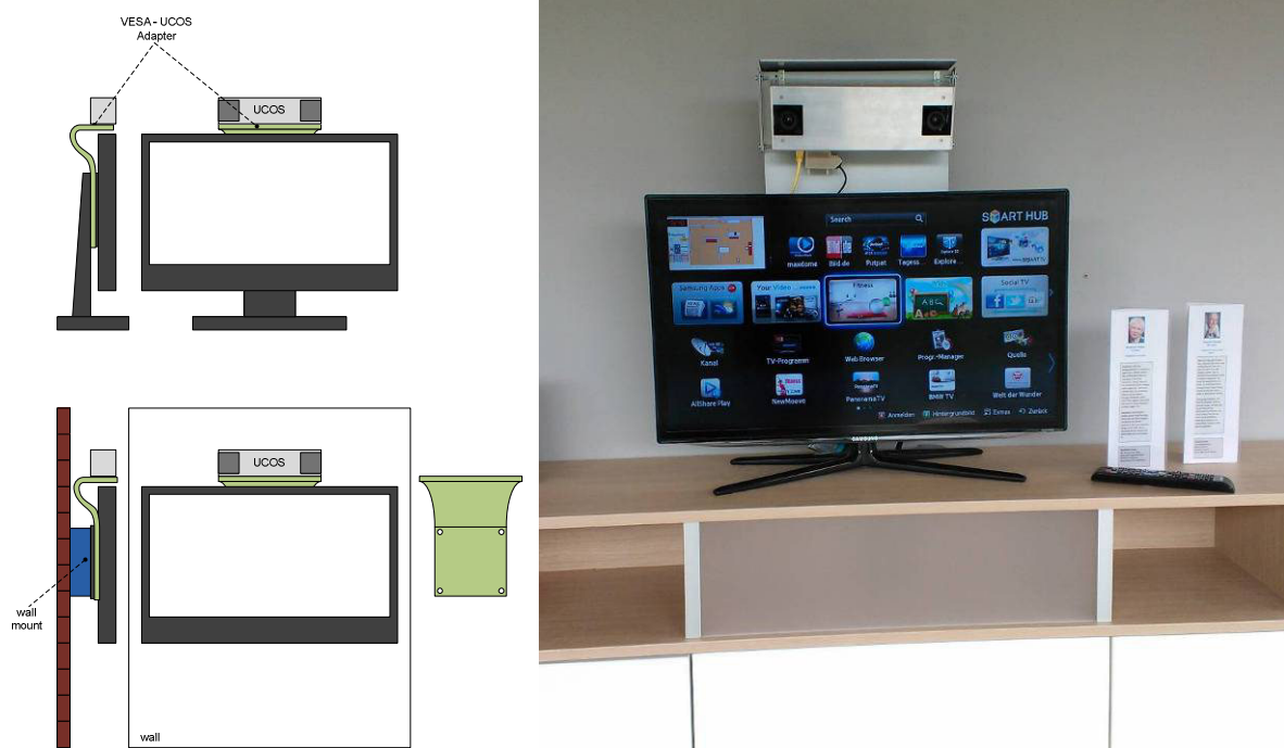
Figure 16: VESA Sensor mounting adapter selected for use in the project.
