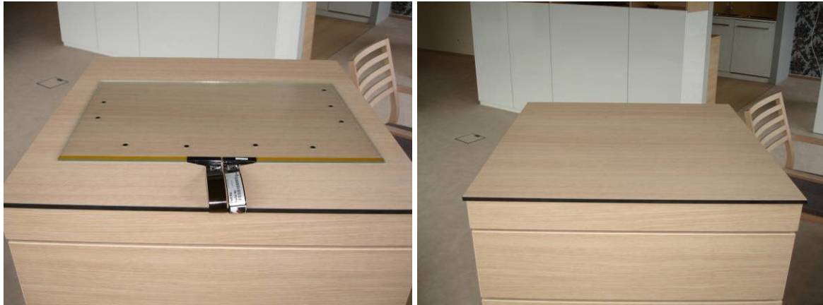
Figure 18: (a) Touch screen for gesture recognition (b) Integration under the wood panel
