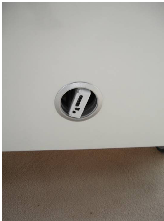
Figure 20: IR sender integrated in the trolley
