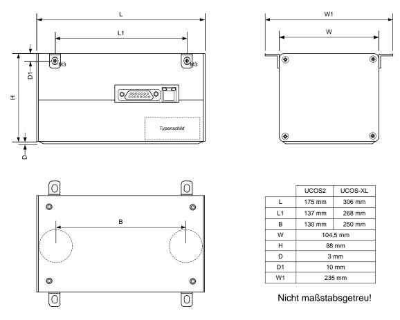
Figure 1. UCOS2XL technical drawing with dimensions in mm.
