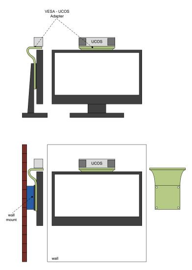
Figure 5. VESA Sensor mounting adapter selected for use in the project.
