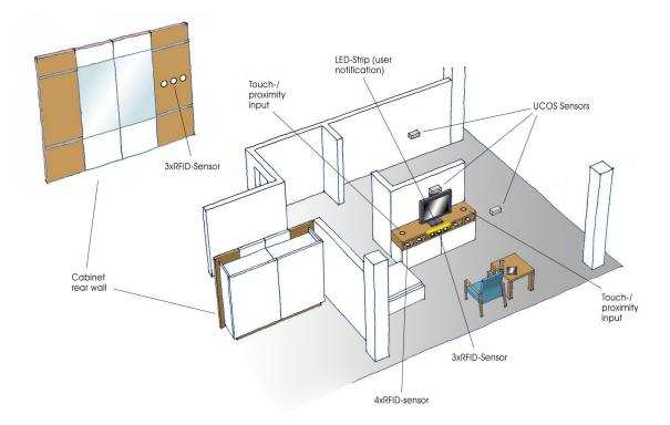
Figure 11: Sensors used in inHaus Service Apartment
