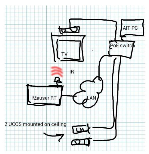
Figure 6. Block diagram of UCOS sensor and other hardware connectivity.
