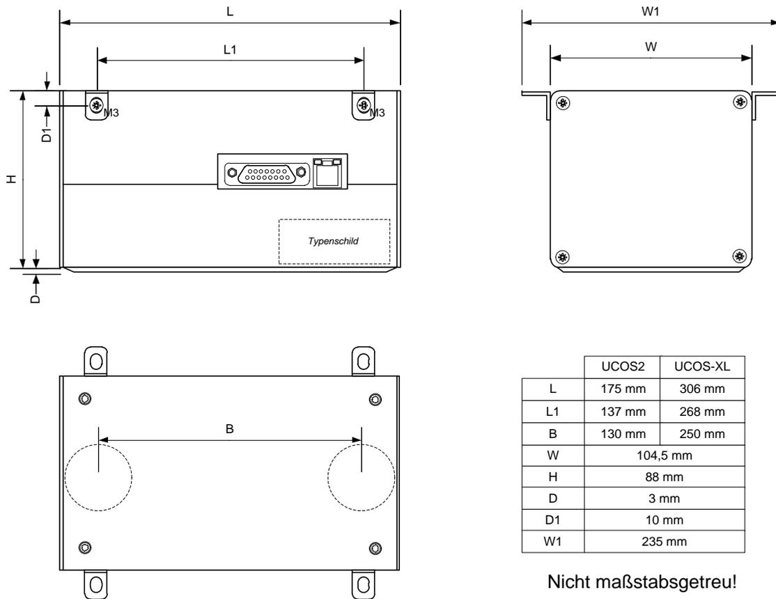
Figure 1. UCOS2XL technical drawing with dimensions in mm.
