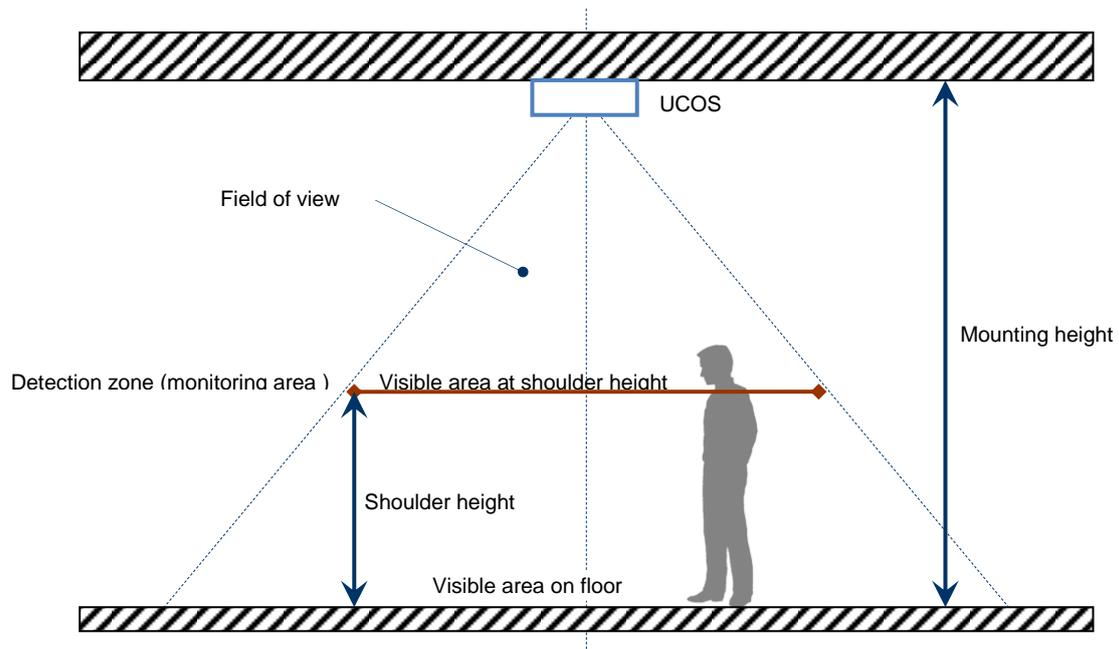
Figure 2. Visualisation of the dimensions in the sensor settings.
