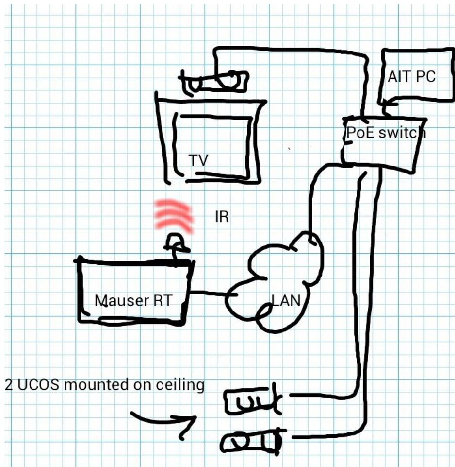
Figure 6. Block diagram of UCOS sensor and other hardware connectivity.
