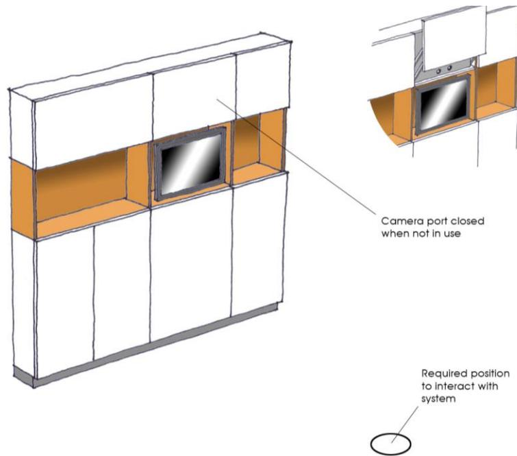
**Figure 4. Fixed Sensor mounting.**
