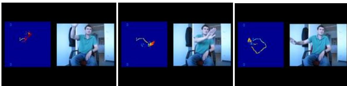
**Figure 1 Sequence of still images of an example of raw hand tracking data from the UCOS2 sensor (left pane) and synchronous video (right pane) for a person performing a "circle" gesture with his right arm.**
