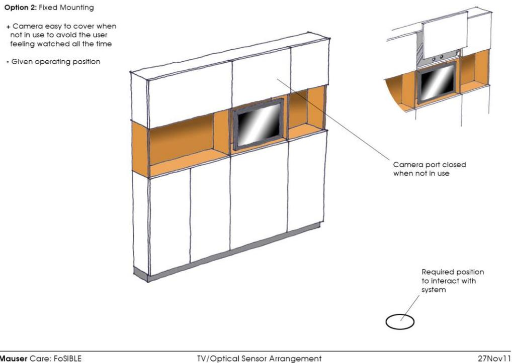
Figure 4. fixed Sensor mounting.
