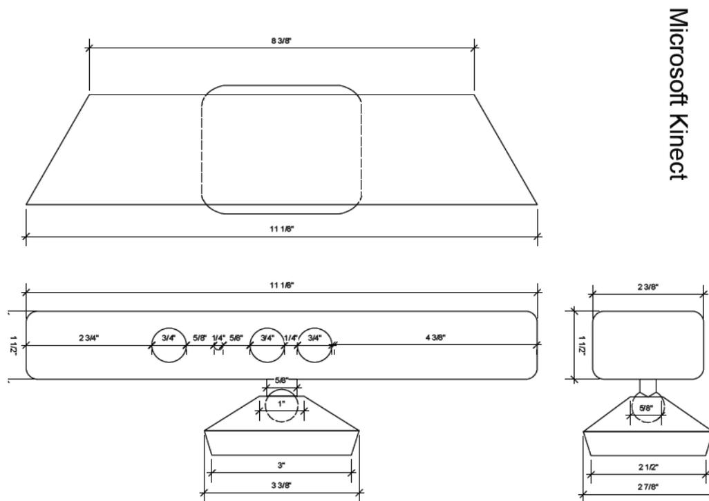
**Figure 1. MS Kinect technical drawing with dimensions in inches (source [6]).**
