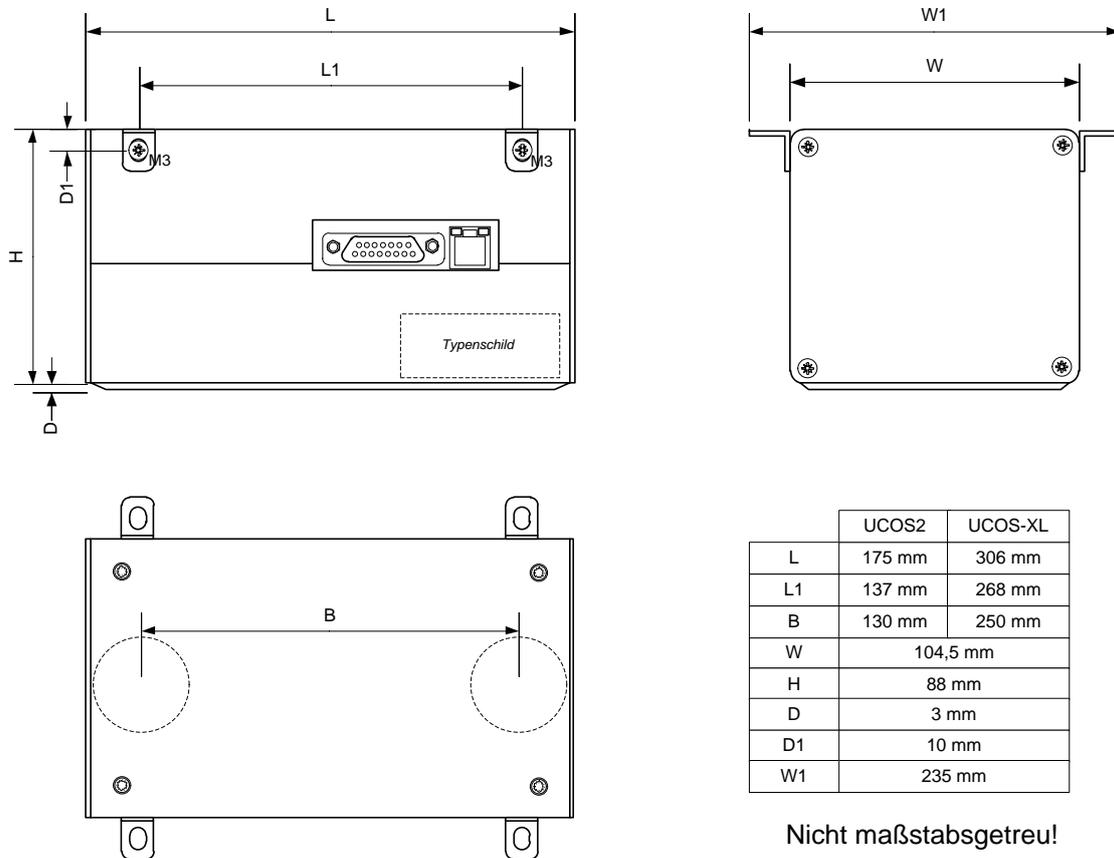
Figure 2. UCOS2XL technical drawing with dimensions in mm.
