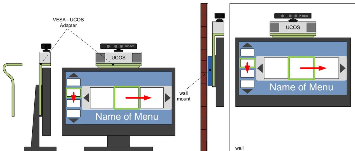
Figure 5. VESA Sensor mounting adapter selected for use in the project.
