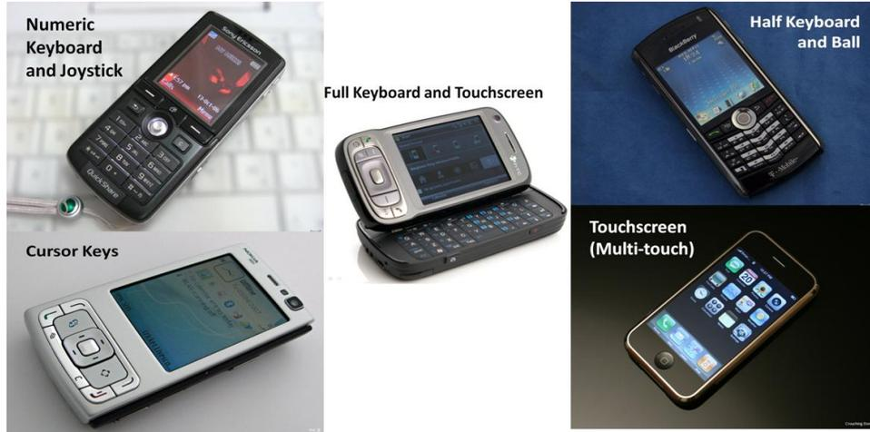
Figure 36. Different input devices
