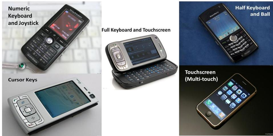
Figure 36. Different input devices
