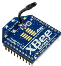
Figure 8 – XBee module configured as ZigBee router
