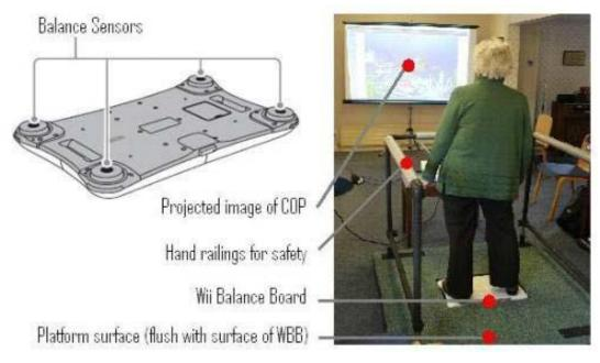
Figure 75 Demonstration of the 'Wii balance board' being operated by an elderly user. The left of the diagram displays the position of the sensors on the board.
