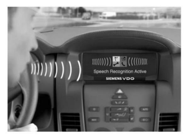
Figure 16 - User interface for voice driven applications in car.
