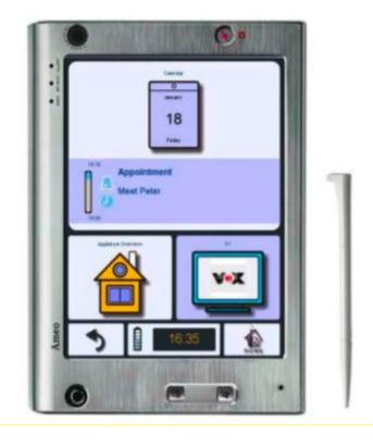
Figure 18 - The i2home user interface for multimodal interaction on a smartphone.
