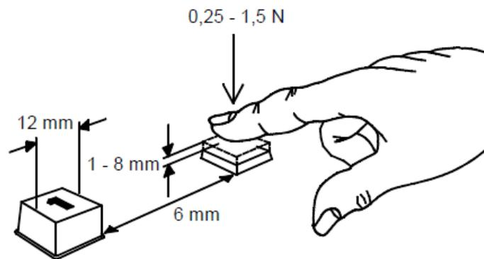
Example of dimensioning for pushbuttons not pressed below the surface
