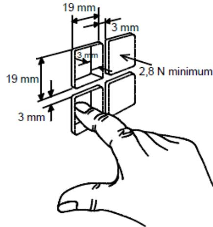
Example of dimensioning for pushbuttons pressed below the surface.
