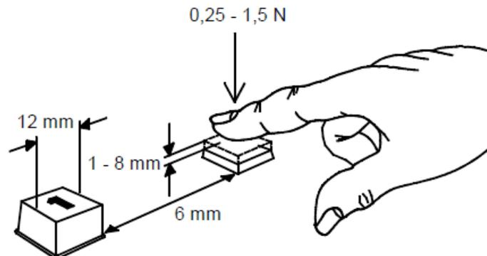
Example of dimensioning for pushbuttons not pressed below the surface
