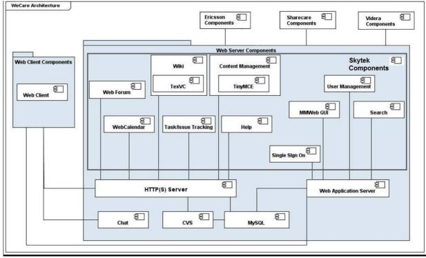
Figure 3 WeCare System Architecture providing a functional overview and showing how different partners components were integrated.
