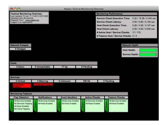
Figure 25 Example of Nagios network monitoring GUI to be used during WeCare pilot utilisation
