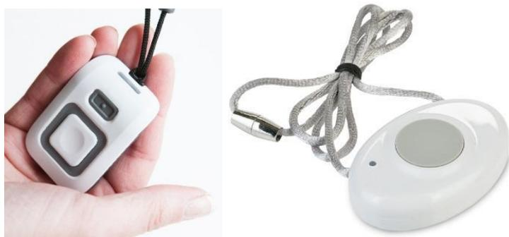
Figure 4. Tunstall fall detection sensor to the left and the Bay alarm fall detection sensor to the right.
