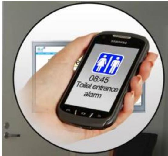
The figure below shows how the system is capable of detecting if the patient laves or enters the room respectively, sending the notification with the exact time.
