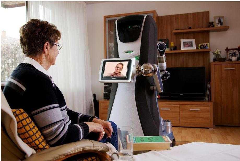
Figure 29. Care-o-bot platform developed by Fraunhofer in Germany.
