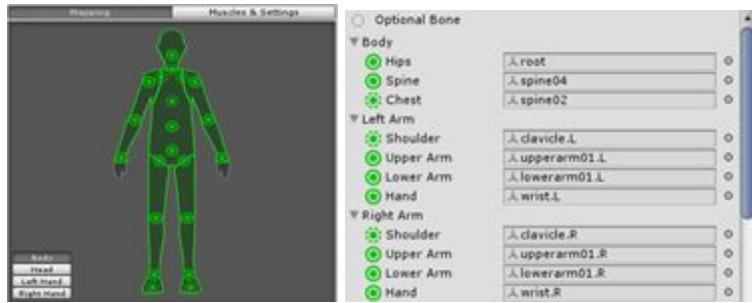
Figure 8 . a) Avatar's skeleton joints. b) Automatic mapping between standard joints and avatar's joint
