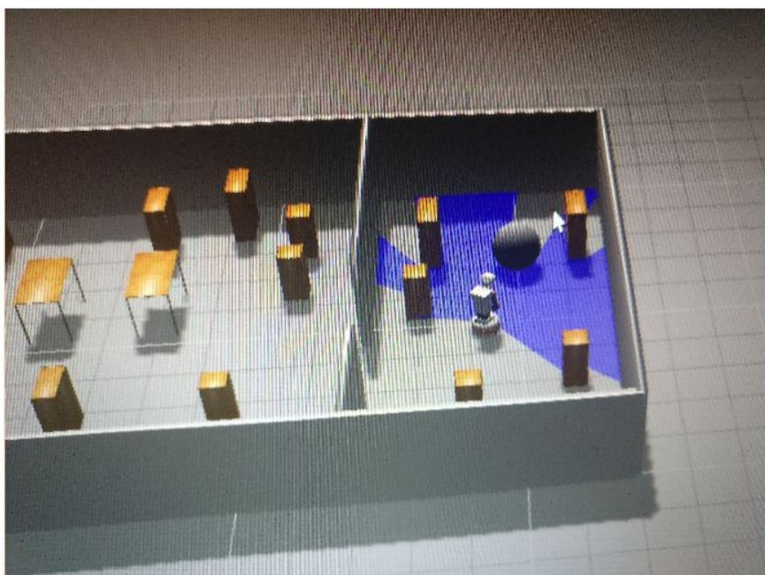
Figure 14 The Gazebo window showing Tiago in an office like environment with dynamic objects represented by the moving sphere.
