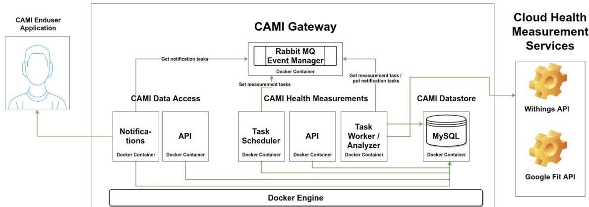
Figure 2 Dockerized CAMI Gateway deployment (showing only Health Measurement, Notification and Storage microservices).
