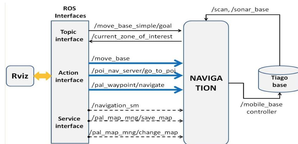
Figure 12 Tiago navigation software architecture
