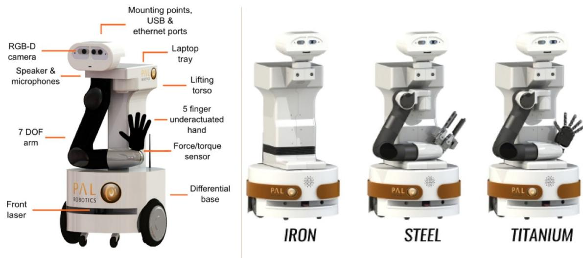
Figure 9 Tiago configuration (left); Iron, Steel and Titanium versions of Tiago.
