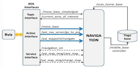
Figure 12 Tiago navigation software architecture
