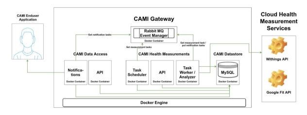
Figure 2 Dockerized CAMI Gateway deployment (showing only Health Measurement, Notification and Storage microservices).
