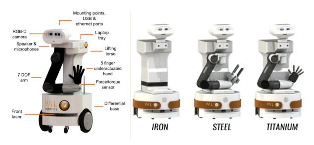
Figure 9 Tiago configuration (left); Iron, Steel and Titanium versions of Tiago.
