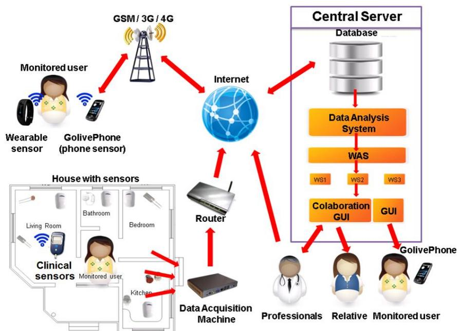
Figure 1 - ENSAFE Integrated System Architecture
