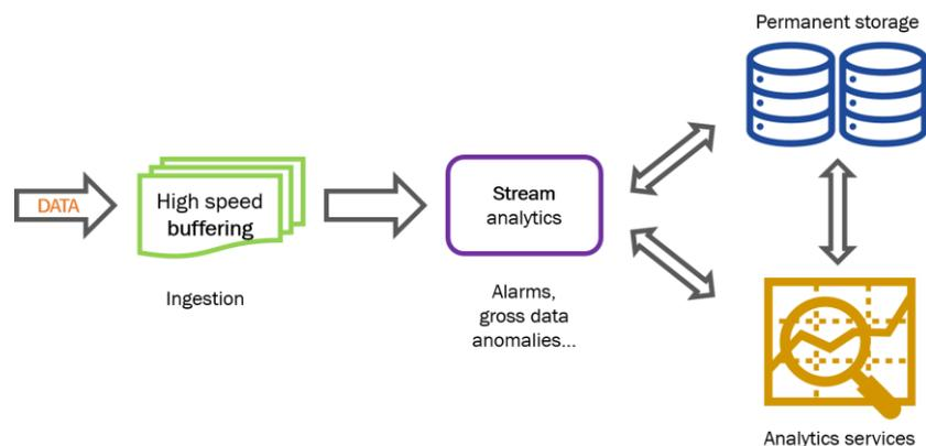
**Figure 1: schematic of the cloud-based architecture**
