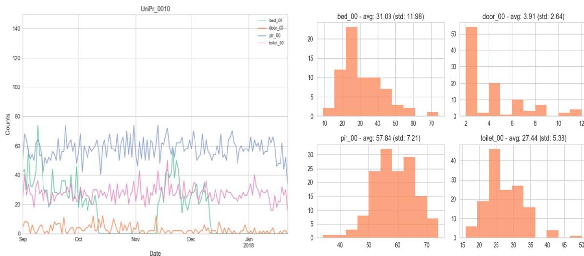
Fig. 2: visualization of daily detected events counts for each sensor (left), and related summary histograms (right).
