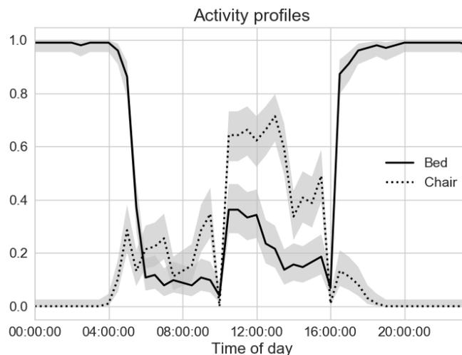
Fig. 4: sensor profiles for bed and chair sensors. Shaded area represent the uncertainty (confidence intervals) in the probability estimate.
