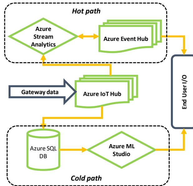
Fig. 1: high-level view of the ENSAFE cloud architecture
