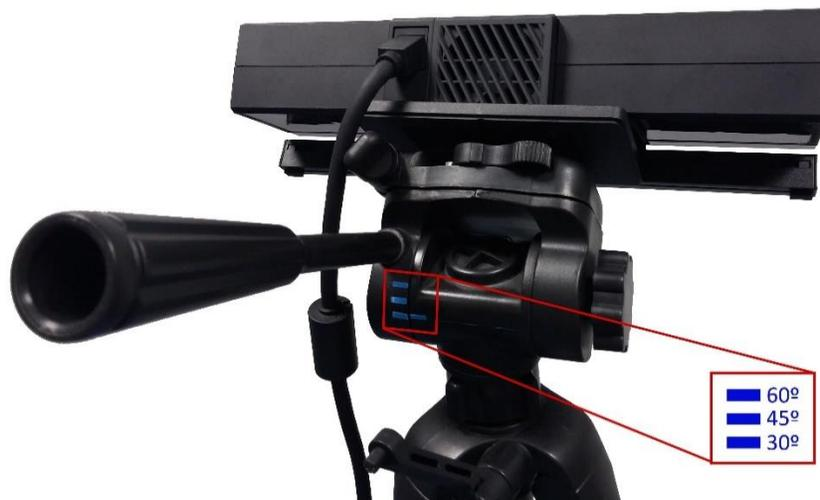
FIGURE 13 – TRIPOD HEAD POSITIONS
