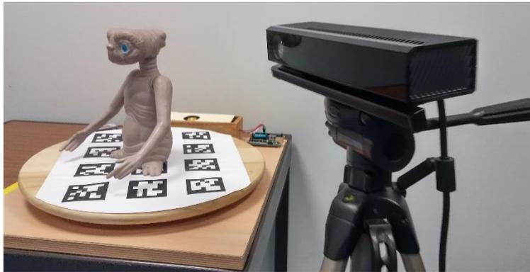
FIGURE 1 - RGB-D SCANNER
