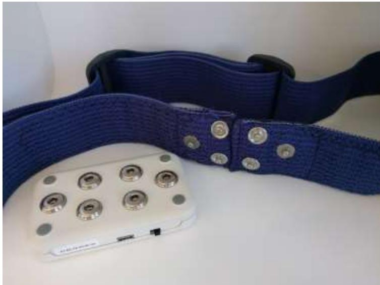
Figure 3 - Snap connectors that allow the textile band to attach to the acquisition unit
