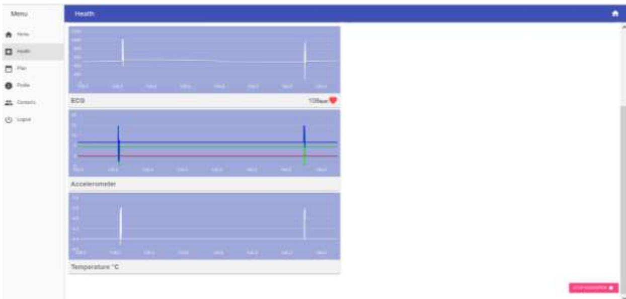
Figure 7 - Health page: Real time sensors acquisition
