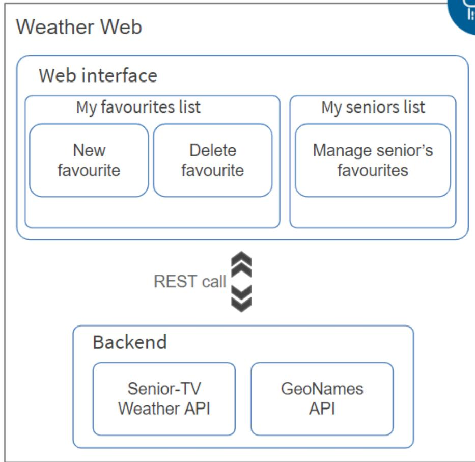
FIGURE 80. WEATHER WEB GENERAL ARCHITECTURE
