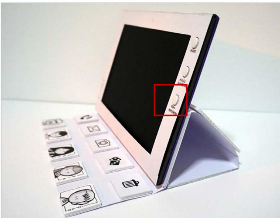
**Figure 04: button for taking a photo and send it to a person**
