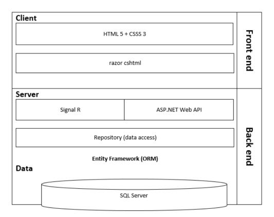
Figure 1 – Architecture Diagram
