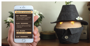
The small social robot tinybots paired with the Sensara sensor network and remote tablet/smartphone.
