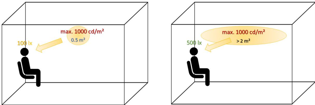
**Figure 11: Sketch showing the  $E_v$  when assuming a luminaire size of  $0.5 \text{ m}^2$  (left) and the luminaire size ( $> 2 \text{ m}^2$ ) when we want to reach the target  $E_v$  of  $500 \text{ lx}$**
