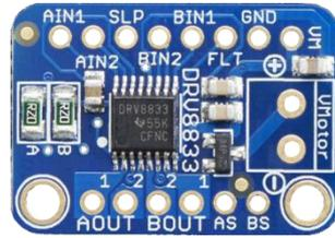
**Figure 52: Adafruit DRV8833 motor driver breakout board.**
