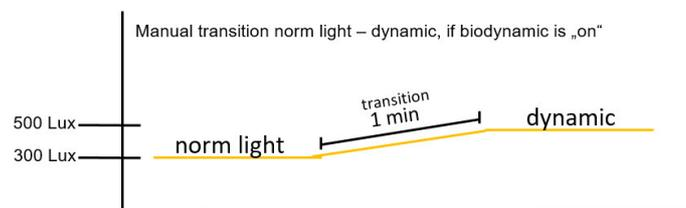
**Figure 8: Course of the manual transition from norm light to biodynamic lighting, if biodynamic lighting is turned on**
