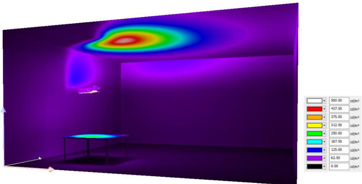
Figure 25: Dialux simulation of the GREAT luminaire showing the luminances in a 25 m<sup>2</sup> room.
