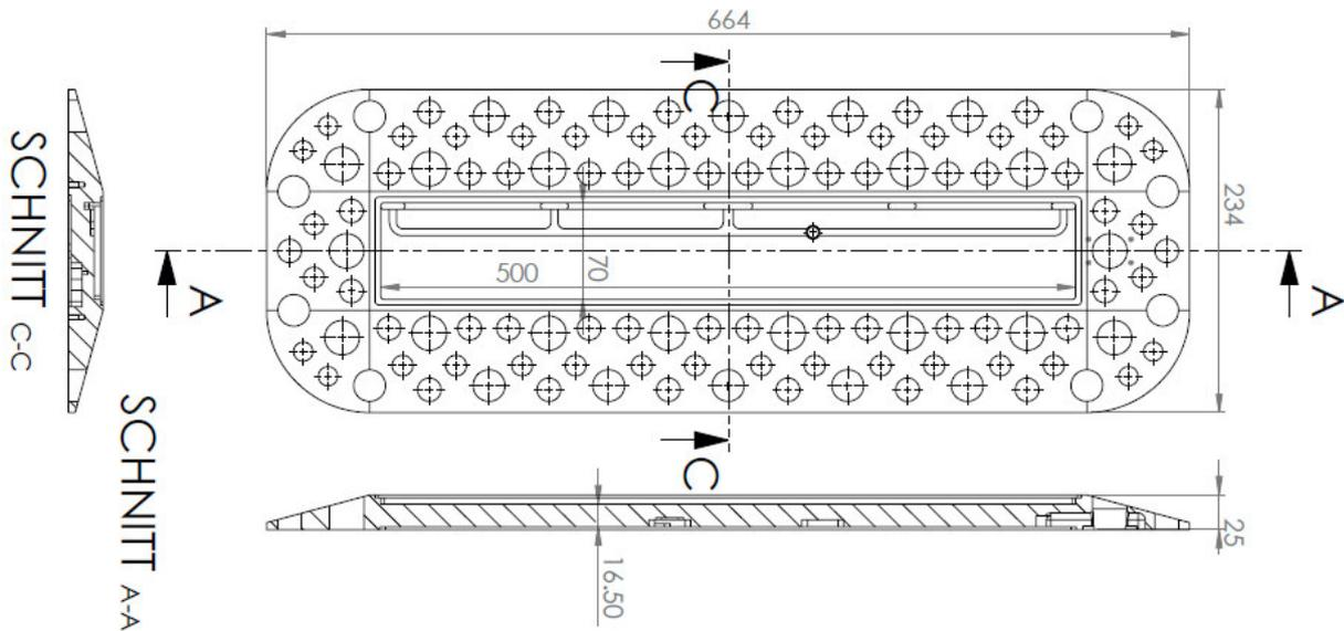
Figure 33: cooling element – realized milled part of Alu
