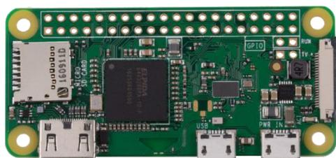
**Figure 51: Raspberry Pi Zero W board computer**
