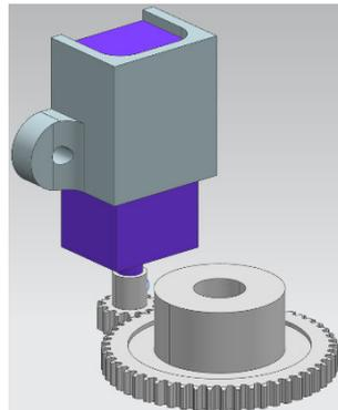
**Figure 45: Motor to gear mechanics**
