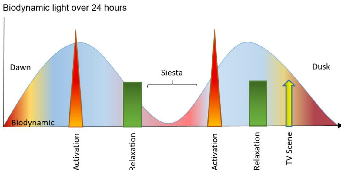
**Figure 2: Schematic representation of the lighting solution in GREAT. Biodynamic light will be a fixed curve, light interventions (activation, relaxation, TV scene) will be adjustable in a timely flexible manner (during a specific time span).**
