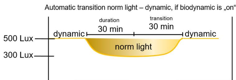
**Figure 7: Course of the automatic transition from norm light back to biodynamic lighting, if biodynamic lighting is turned on**
