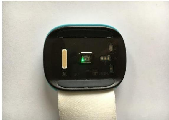
**Figure 62: Everion back with light and galvanic skin sensors**
