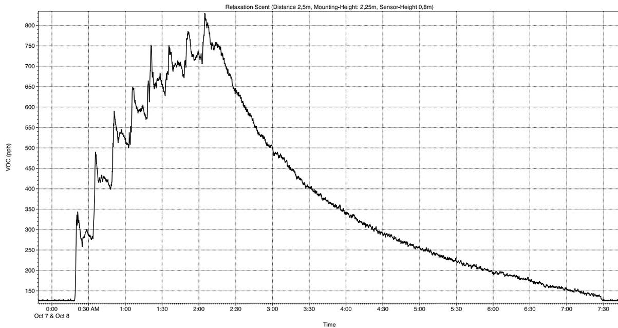
**Figure 58: VOC level builds up with every dispense. A delay between 1-5 minutes can be observed.**
