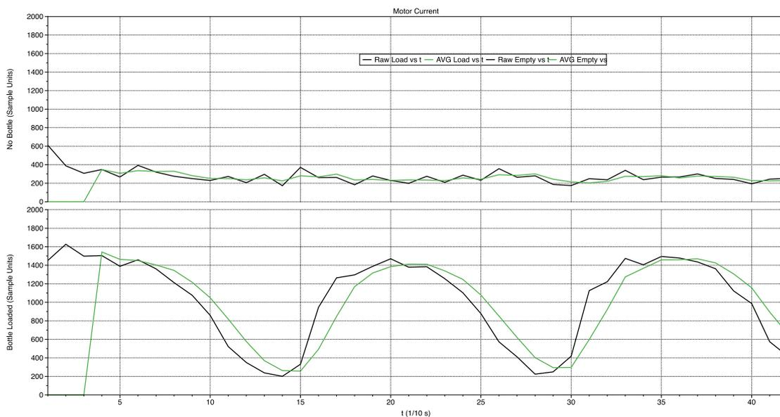
**Figure 54: Current flow to motor during pump cycles with no bottle inserted (top), and bottle inserted bottom) as raw signal and smoothed signal.**
