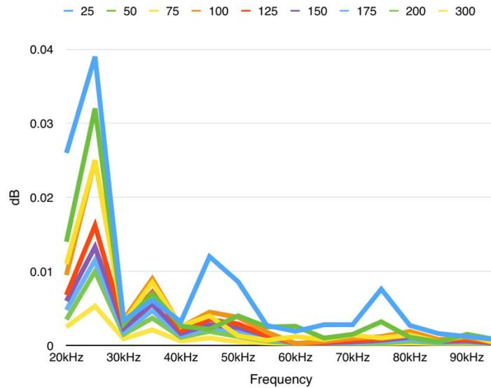
**Figure 35: Drop-off of signal level depending on frequency and distance**
