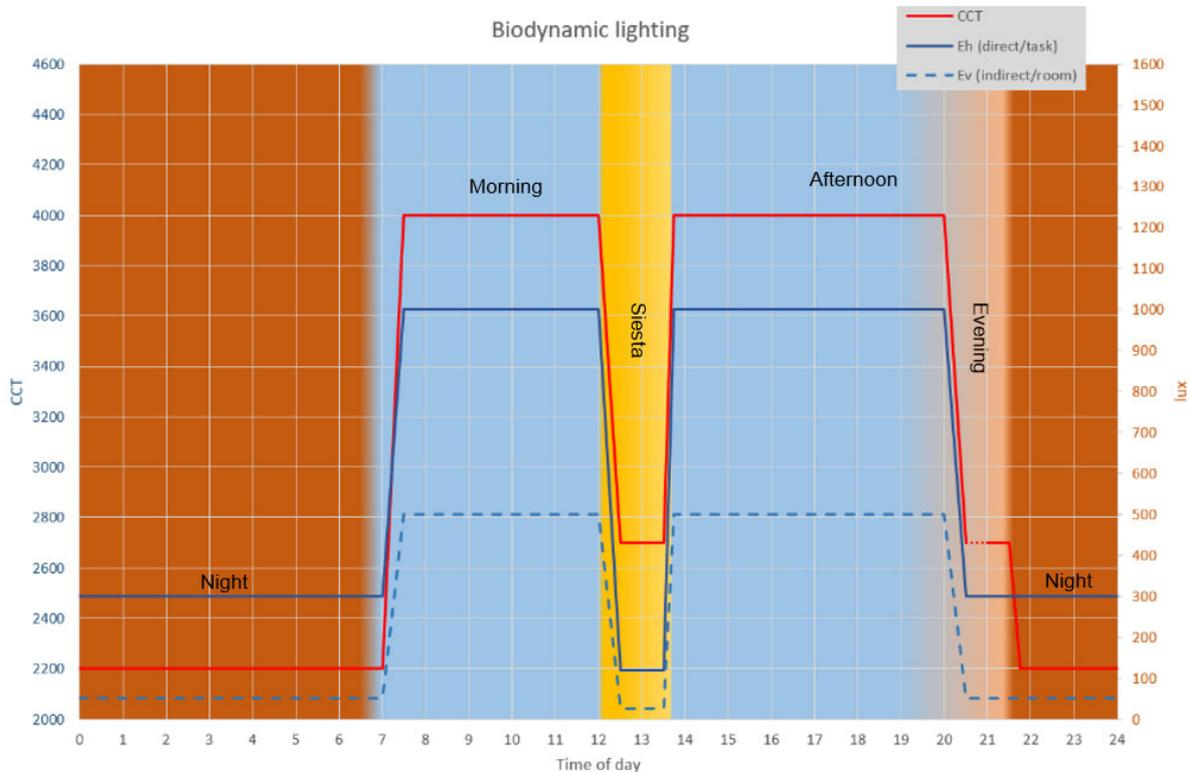
Figure 3: Biodynamic lighting concept. CCT...colour temperature in Kelvin, Eh...horizontal illuminances of the task light, Eh<sub>Room</sub>...horizontal illuminance of ambient room light (resulting from Ev + Eh Task, for clarity reasons Eh<sub>Room</sub> is not shown), Ev...vertical illuminance at the eye level
