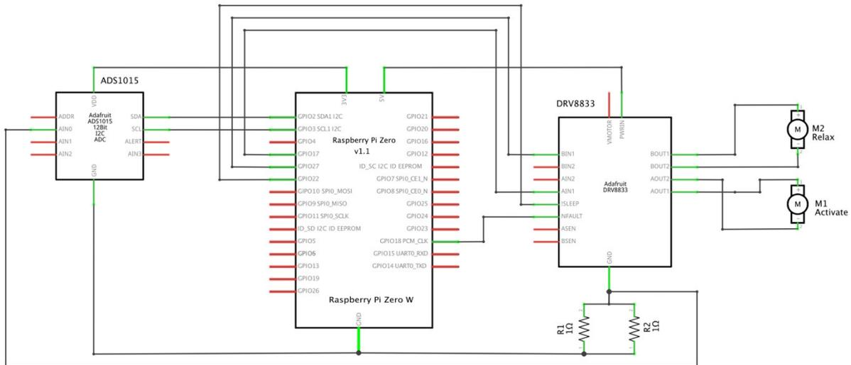
**Figure 55: Schematics for the electrical components of the scent module.**
