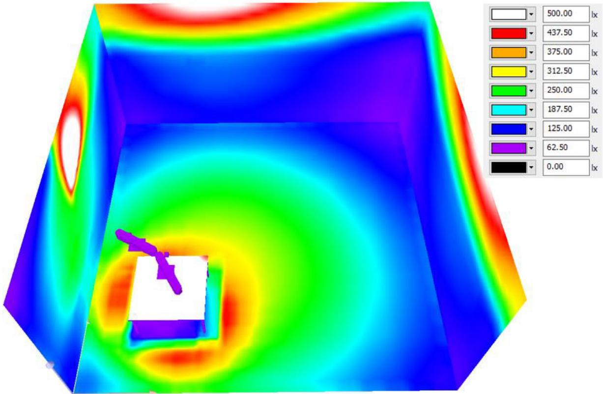
Figure 24: Dialux simulation of the GREAT luminaire showing the illuminances in a 25 m<sup>2</sup> room.
