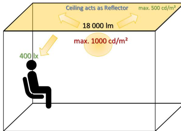
**Figure 12: Indirect illumination concept for the GREAT luminaire (Uplight)**
