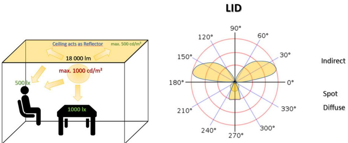
Figure 15: Finalized lighting concept for the GREAT luminaire
