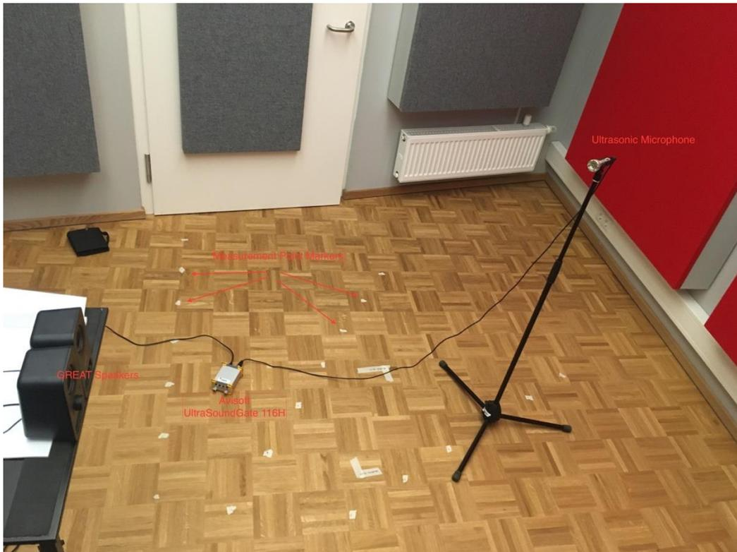
**Figure 34: Sound measurement setup in Audio-Lab at FHV.**
