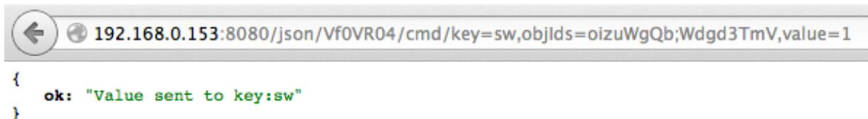
Figure 18: Example cmd request to switch two lighs on
