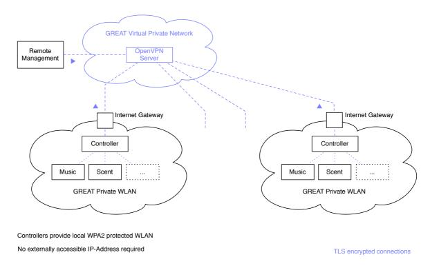
Figure 3: Distributed GREAT installations connected over VPN.
