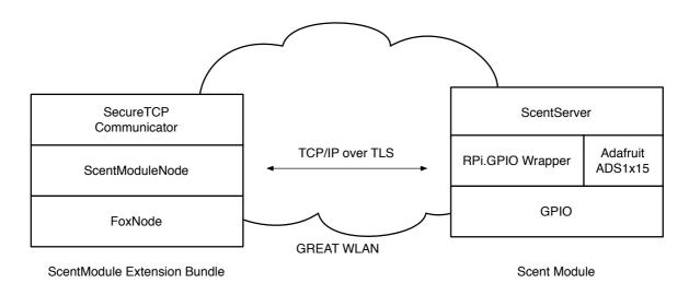
Figure 25: Integration of the scent module into the GREAT controller system based on Intefox.
