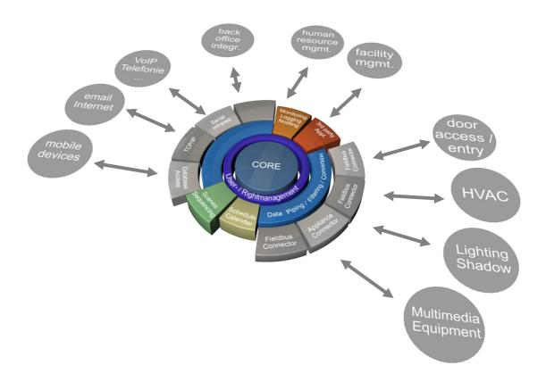
Figure 6: Basic architecture of the foxcore server
