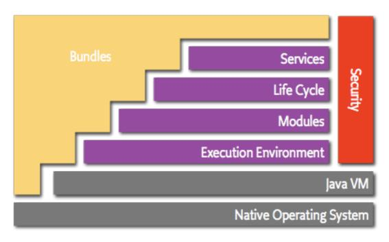
Figure 4: OSGi Architecture Diagram, Source: OSGi Alliance, https://www.osgi.org/developer/architecture
