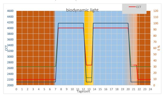
Figure 19: Example biodynamic light definition
