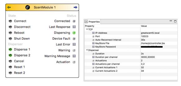
Figure 26: Input and output events (left) and parameter settings (right) of the scent module extension.
