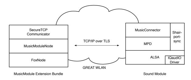
Figure 23: Communication between the Intefox music module extension and the sound module.
